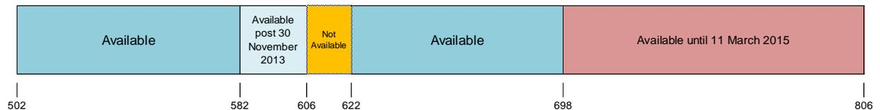
**Figure 1:** Shows the changes affecting radiomicrophones.
